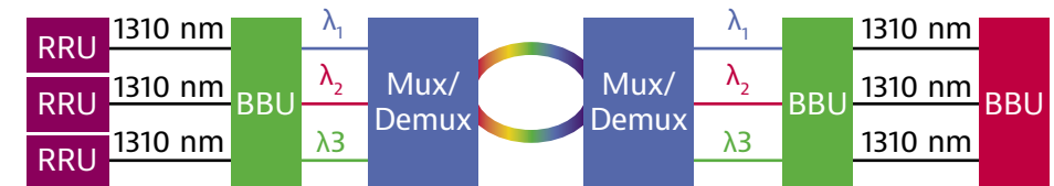
Figure 3.6 Enhanced multiplexing with wavelength conversion
