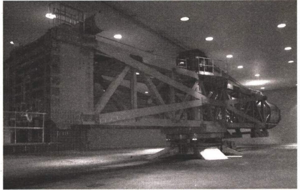
Hold On! —IEEE member Ken Innes (left) attempts to grasp a power connector while wearing bulky astronaut gloves. The power unit is identical to a replacement unit installed in HST and was used in the High Bay Clean Room to train astronauts for the repair mission. Goddard's 120-foot-diameter centrifuge (above) can accelerate a 2.5 ton payload up to 30 Gs, well beyond the force experienced during a launch.
