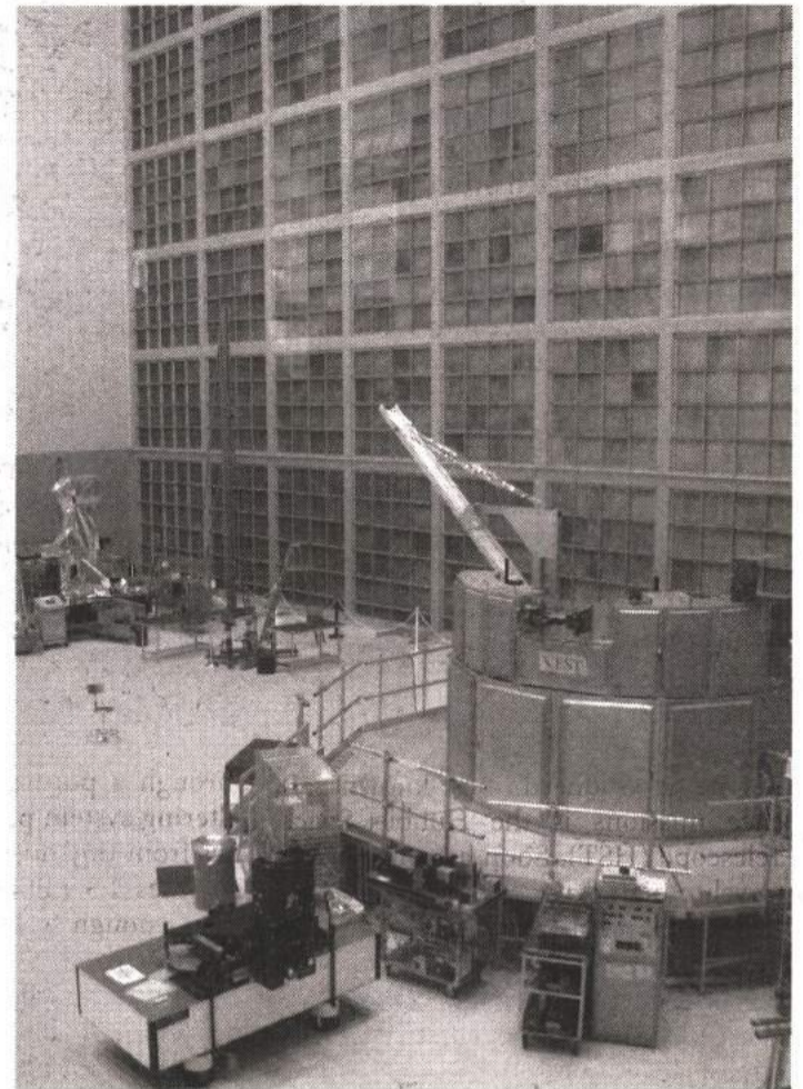
NASA Scale —Tour participants (left) gather in front of Goddard's largest thermal vacuum chamber. Engineers use the chamber to subject spacecraft to the extreme heating and cooling cycles that will be encountered in the vacuum of space. Goddard also has the world's largest clean room (right), most recently used to assemble and test hardware for the upcoming Hubble Space Telescope repair mission. The wall of filters at the right cleanses incoming air of tiny dust particles.
