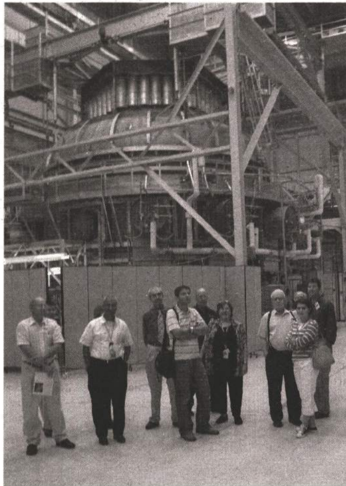
NASA Scale —Tour participants (left) gather in front of Goddard's largest thermal vacuum chamber. Engineers use the chamber to subject spacecraft to the extreme heating and cooling cycles that will be encountered in the vacuum of space. Goddard also has the world's largest clean room (right), most recently used to assemble and test hardware for the upcoming Hubble Space Telescope repair mission. The wall of filters at the right cleanses incoming air of tiny dust particles.
