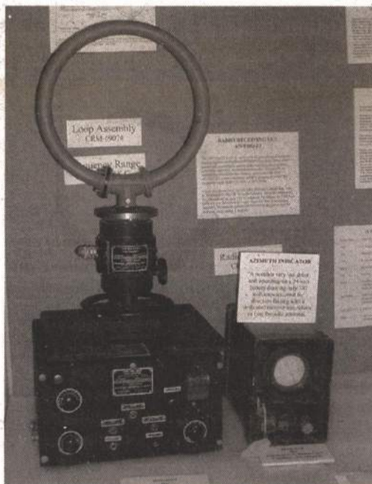
A WWII radio direction finder set comprised of CRM-69014 loop antenna, CRM-46153 receiver and the IP-740/GR azimuth indicator.
